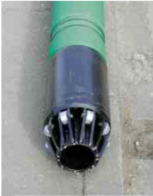
Guiding sleeve with gliding rollers (Patent pending)
